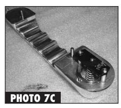
**7.** Place the two plastic spacers into position and place the spring over the push rod. Now place the plastic mounting clip back into position (See Photo 7A). Align the two supplied phillips head screws through the plastic mounting clip and spacers and tighten with a screwdriver (See Photo 7B & 7C).
