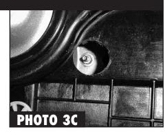
3. You can either use a hole saw, drill bit, or snips to make the hole for access to the nut that needs to be removed (See Photo 3A & 3B). A 1/2" hole is the minimum that you will need to make. Doing an oversized hole will make the next step much easier. You should now be able to see the nut (See Photo 3C).
