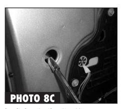
8. Place the billet handle back into position on the door (See Photo 8A) and put the factory nuts back onto the studs and tighten (See Photo 8B & 8C).
