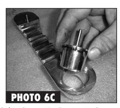
6. To start the reassembly, put the plastic spacer over the new push button and make sure that it is aligned with the four indentations (See Photo 6A & 6B). Then insert into the billet handle (See Photo 6C).
