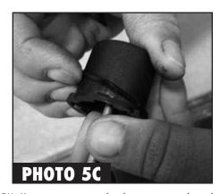
5. With the handle face down on a workbench, remove the two torx screws with a T-10 torx driver (See Photo 5A). You can now remove the plastic mounting clip and spring from the factory handle (See Photo 5B). Now take out the push button and remove the plastic spacer (See Photo 5C).
