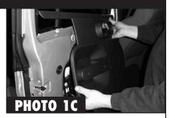
**Rear 1.** Begin by removing the two phillips head screws from the door panel (See Photo 1A). Now remove the door panel by pulling outward from the bottom (See Photo 1B). Once all of the clips are pulled out, lift upward to release the door panel from the door (See Photo 1C).
