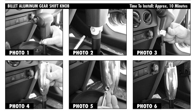
Begin by twisting the bottom boot of the shifter clockwise (Photo 1). Remove the torx head screw with a t-20 torx (Photo 2) and pull the stock shifter off (Photo 3). Place your new Billet shifter back in place (Photo 4). Align the set screw back up and tighten (Photos 5 and Photo 6).
