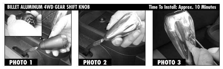
Begin by setting the parking brake, placing the transmission in natural, and put the transfer case in natural or 4lo. With a firm pull, the stock shifter will come off (Photo 1). Place your new Billet Shifter into place and align for the set screw (Photo 2). Insert the set screw into the V-shape portion of the shaft and tighten (Photo 3).
