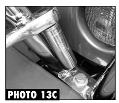
**13A, 13B & 13C.** Using a 1/2" bolts, star washers and flat washers on each side, tighten down the grille guard. (See Photos 13A, 13B & 13C)
