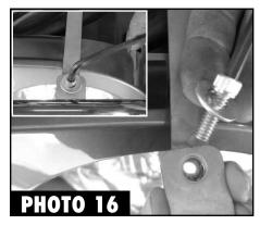
**16.** Insert the 1/4''-20x3/8'' allen head screw through the bracket and into the strap and tighten. (See Photo 16)
