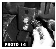
**14.** Now securely tighten the two previously fingered tightened bracket bolts on each side. (See Photo 14)
