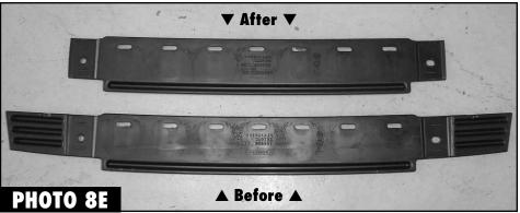
**8.** Measure and mark on both sides of the plastic bumper spacer plate 3-1/4" from the inside kick out. (See Photos 8A & 8B) Using a cutting tool make both cuts at the marked line. (See Photos 8C & 8D) This is a before and after of your bumper spacer plate. (See Photo 8E)
