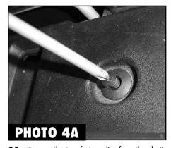
**4A.** Remove the two factory clips from the plastic bumper spacer plate located just behind the front bumper and right in front of the factory grille location. (See Photo 4A)
