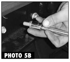
**5.** Towards each corner of the bumper there are two nuts and bolts that need to be removed. (See Photo 5A) Remove all four with a 15mm socket. (See Photo 5B).
