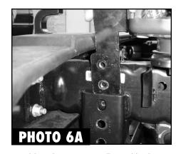
**6.** Slide in the appropriate grille guard bracket into the slot located along the frame rail. (See Photos 6A & 6B)
