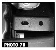
**7.** Using the supplied 1/2" bolts and lock washers, finger tighten them into the brackets. (See Photo 7A) Repeat for the other side. (See Photo 7B)
