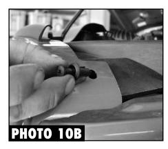
**10.** Place the grille back into position and snap in the lower clips (See Photo 10A), then place the six upper clips back into place. (See Photo 10B)
