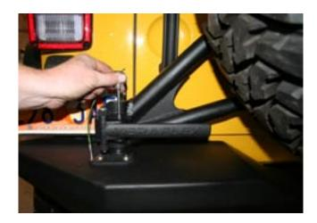
The final step is to install the pivot bushing grease zerk and then tighten all the mounting bolts and bracket bolts. Tighten the bolts in a criss-cross pattern so the pivot and fixed brackets don't move out of place. Check the proper movement and alignment of the carrier several times as you finalize the installation.
