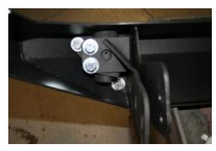
Next assemble the fixed post end, again leaving the bolts loose until the final adjustment is made. Install the polyurethane cover sleeve on the fixed post.
