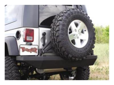
The JK RockGuard Spare Tire Carrier includes a multi-plane adjustable mounting bracket that must be installed inside the rear bumper before the bumper is installed on the JK. The TeraFlex Tire Carrier will only work with a TeraFlex RockGuard rear bumper p/n 4654100.
