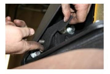
The tire mount is set for 5 on 5 lug pattern for the stock JK wheels. Wheel adapters are available from TeraFlex for other wheel lug patterns.
