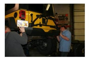
The top rail of the tire carrier should line up with and slightly compress the urethane bump stops on the tailgate when the latch is closed.
