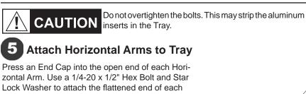
Press an End Cap into the open end of each Horizontal Arm. Use a 1/4-20 x 1/2" Hex Bolt and Star Lock Washer to attach the flattened end of each Horizontal Arm to the bottom of the Tray. Use a 1/4-20 x 1-1/2" Hex Bolt and a Star Lock Washer to attach the other end of each arm to the Tray.
