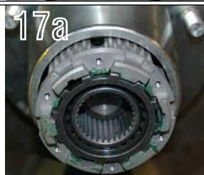
17a -Slide the lockout hub body into the wheel hub. You may have to slightly rotate the hub to get the splines located.
