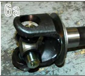
6a -Install the mud slinger (Item B) onto the stub shaft as shown. The ujoint can also be prepped for assembly by removing the caps and placing the joint in the shaft.
