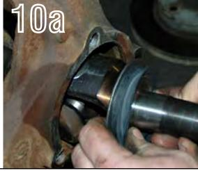
10a -Slide the V lip Seal over the mud slinger as shown. Apply a thin film of grease on the lip.
