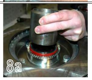
8a -Once the shafts are assembled, the outer spindle bearings can be greased. The kit already has the inner bearing greased as well as the hub seal installed. For future reference this photo shows the proper way to install the seal. Pay close attention to not damage the reluctor wheel teeth.
