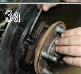
Us a 5 mm hex key to remove the screw from the sensor, but do not remove the sensor at this time as it may be damaged. Carefully tap on the unit bearing to seperate it from the knuckle. Pay close attention to not ruin the metal dust shield as this will be reused. Once the bearing is seperated from the knuckle, remove the sensor by pulling it straight out.
