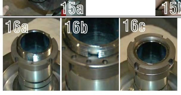
Before going into the installation of the spindle nuts onto the spindle. Look closely at the configurations to the left. 16a shows the nut with the pin facing toward the outside of the vehicle. This is so the tab washer in 16b can lock the nut in place keeping in from turning. 16c is simply a jamb nut pinching the nut washer assembly together.
