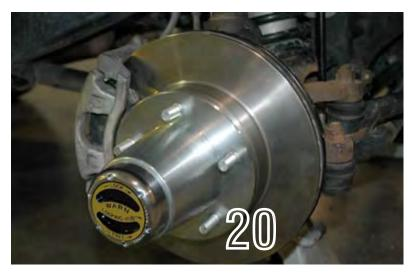
20 -The Spyntec assembly is complete at this time. You are ready to place the wheel on and torque down the lugnuts. Make sure you retorque the lugnuts after 50 miles as well as after heavy offroading.
