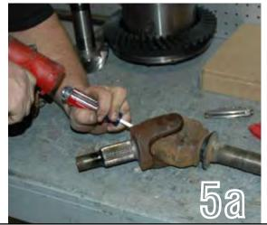
5a -Using a small screw driver and hammer, tap the ujoint retaining clips from the inner axle shaft.
