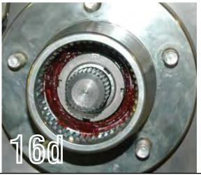
16d- Thread the inner spindle nut onto the spindle. Using a spindle nut socket and torque wrench, tighten the spindle nut (photo 16a) to 50 ft-lbs. Do not over tighten the nut. Rotate the hub back and forth while tightening. Back off the spindle nut 1/4 turn. Slide on the lock washer (photo 16b). Make sure the pin is aligned with a hole on the nut. Thread the outer nut onto the spindle and torque to 125 - 150 ft-lbs.
