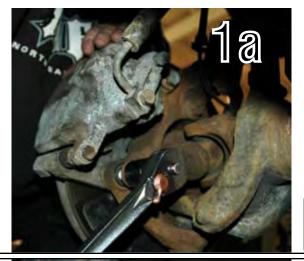
1a- After the wheel is unbolted, the brake caliper will need to be removed. A 21 mm socket or wrench will be needed.
