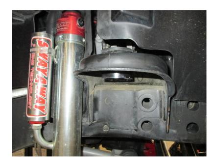
13. Remove upper lock ring from the bumpstop, slide it up from the bottom and re-install lock ring with the included
