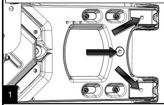
Position the mount and start the M8 bolt(7) and washer(8) into the mounts upper left hole, spacer(10) will go between the mount and carrier, leave bolt loose. Note: If there is a problems starting the M8 bolt, test fit spacer and bolt, without mount, to move nut into position. Next tighten the left bolt to keep plate in position, then remove spacer and M8 bolt, install as before.
