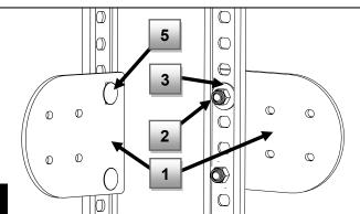
The RotopaX Mount can also be mounted directly to the Hi-Lift Mount by installing two 1/2 x 1.25" carriage bolts(4) through the RotopaX Mounts square holes and Hi-Lift Mount top two outer most holes. Each bolt gets a washer(3) and nut(2). Tighten nuts to 55 ft-lbs.
