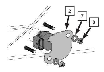
NOTE: SENSORS NEED TO BE INSTALL IN THE SAME ORIENTATION AND POSITION THAT THEY CAME OUT OF OEM BUMPER
