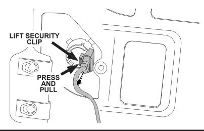
NOTE: USE A TABLE TO HOLD BUMPER WHILE REMOVING HARNESS
