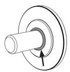
Install O Ring onto endcap before installing onto the Sway Bar.
