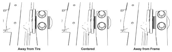
Cycle the rear suspension to ensure the sway bar arm and link are not rubbing.
