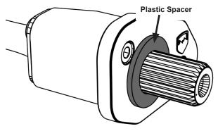
Spacers can be configured to set the arm closer to the frame or the tire depending on your needs. Put the arm away from the tire (closer to the frame) unless it will rub on an aftermarket inner fender liner.
