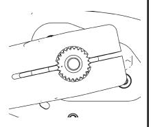
Make sure the gap in the arm alings with the dot on the bar.
