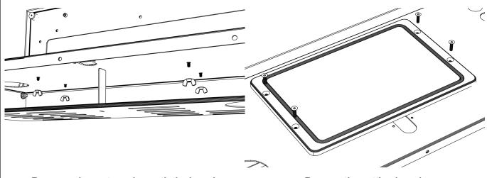
Remove wing nuts underneath the board.
