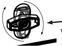
Rotate to lock or unlock
