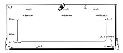
In case there is some confusion, here is a diagram showing which hole on the backing plate goes with which vehicle.
