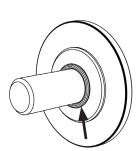
Install O Ring onto end cap before installing onto the Sway Bar.
