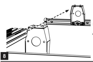
Slide the cross bar along the top of the brackets so the t-nuts go into the grooves on the bar.
