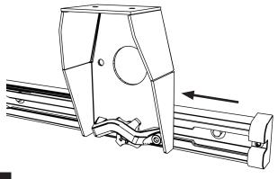
The bracket's position must be the same on both sides of the bed.
