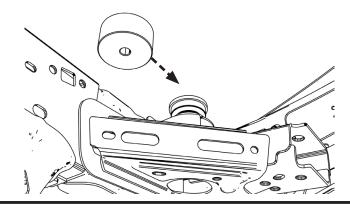
Lower the body back onto the spacer after they have been installed.
