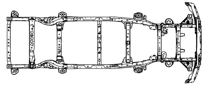
THE BODY LIFT CAN BE INSTALLED IN ANY ORDER (FRONT TO REAR, LEFT TO RIGHT, ETC.) WHAT IS IMPORTANT IS THAT SOME OF THE BOLTS REMAIN THREADED INTO THE HOLES AT ANY GIVEN TIME.
