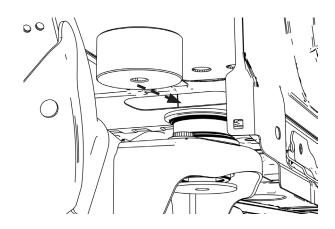
Lower the body back onto the spacer after they have been installed.
