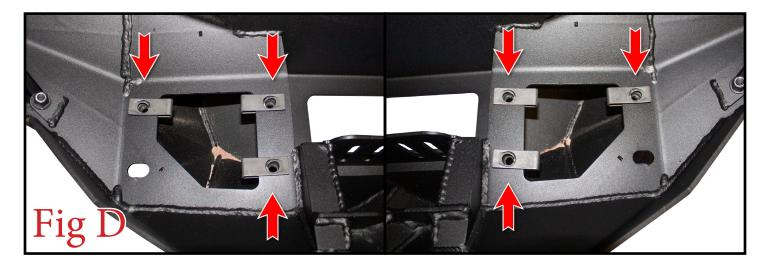
7. Set the bumper in place on the vehicle. Loosely install the supplied 3/8" Bolts (x6) and 3/8" Washers (x6) into newly installed U-nuts from the back side of the vehicle's frame horns. Then, install the supplied 1/2" Bolts (x2), 1/2" Washers (x4), and 1/2" Lock Nuts (x2) into the lower/outer mounting hole on each side. (Fig E)
