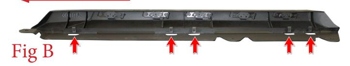
5. If you have any lights to install in your Side Steps, now is a good time to do so. To mount your rock lights, you will have to remove the side panels. To do this, you will need to use a 7/32" Allen Wrench or Allen Socket and a 9/16" Wrench to remove both mounting bolts. Once your lights are installed, set the panel back exactly as it sat before you took it off and reinstall both mounting bolts. Please follow the light manufacturer's guide for mounting/wiring information.
