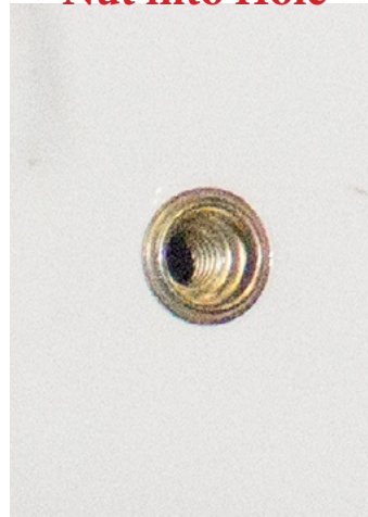
Push Rivet Nut into Hole
