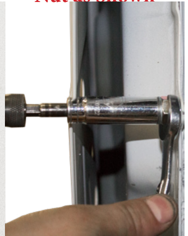
Tighten Rivet Nut as Shown
