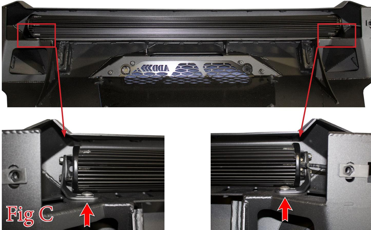
5. Tilt your light to your own preference. Then, tighten the light's mounting bolts to the light manufacturer's torque specification.
