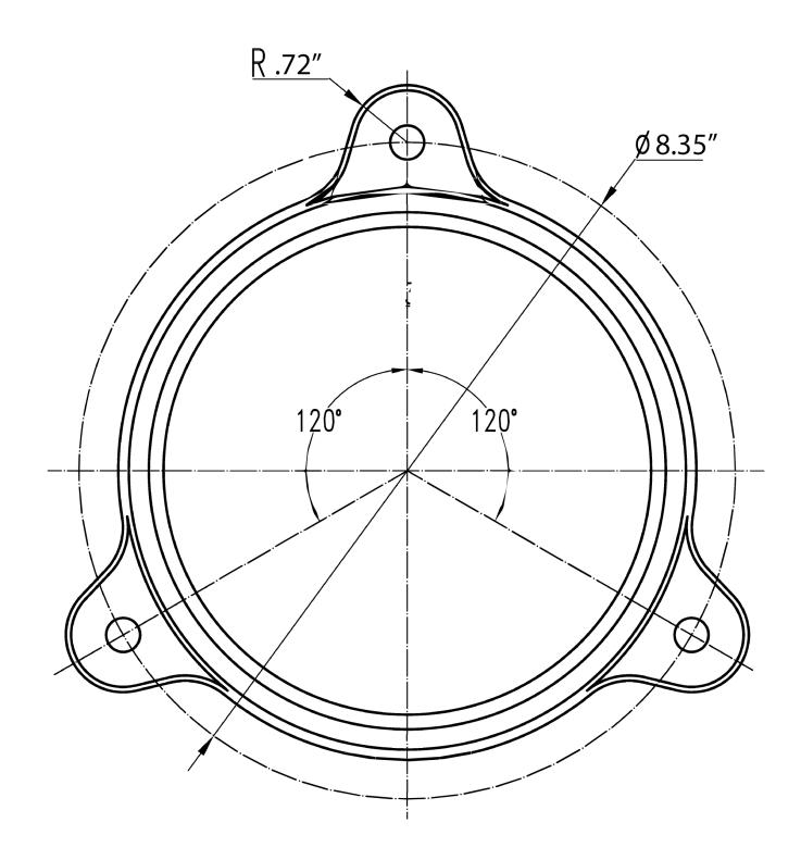
To Scale. For reference only Do not drill holes into the work table until you have received your vise and marked the holes using the mounting tabs on the vise.
