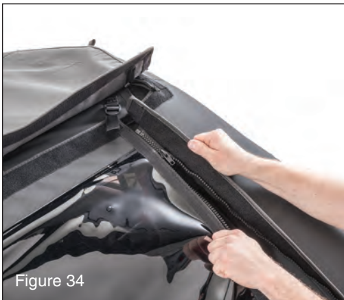
Start rear window zipper to side window as shown. Do not zip all the way at this time. (see FIG 34)
