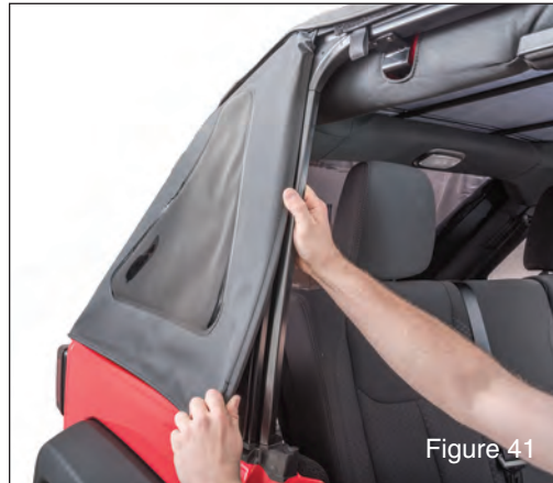
Figure 41 Begin to secure the windows by starting with the vertical lip on the side windows as shown. (see FIG 41)
