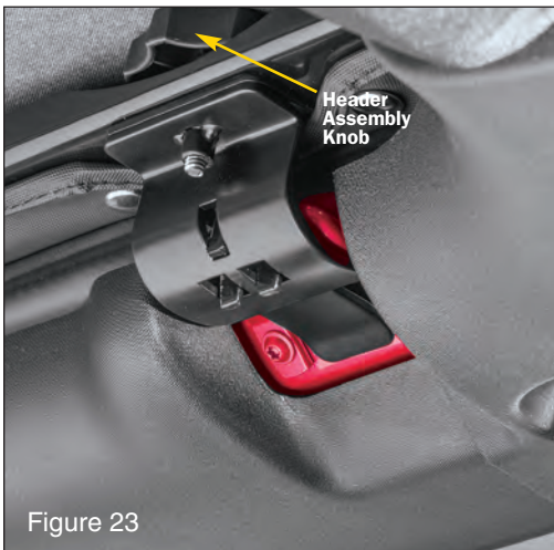
Figure 23 Secure the Header Channel to the vehicle using the plate and the knob removed in FIG 19. (see FIG 23)
