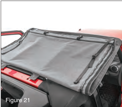
Figure 21 Place header channel with soft top onto vehicle. (see FIG 21)
