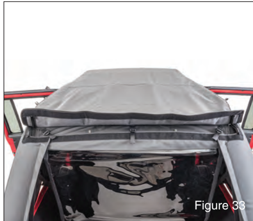
Install rear window to the 3 straps at rear of top. (see FIG 33)
