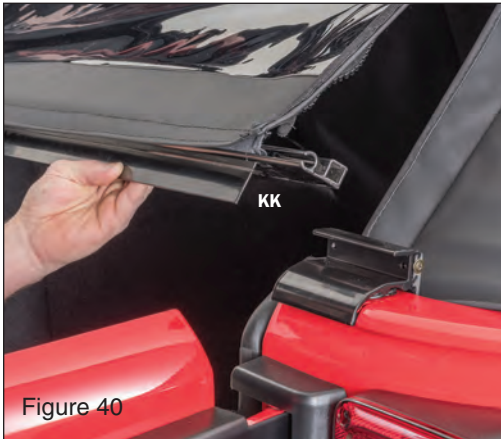
Figure 40 Slide the Rear Window Tailgate Bar (KK) onto the Rear Window as shown. Note orientation carefully. Insert the Tailgate Bar into the Tailgate Bar Retainers. (see FIG 40)
