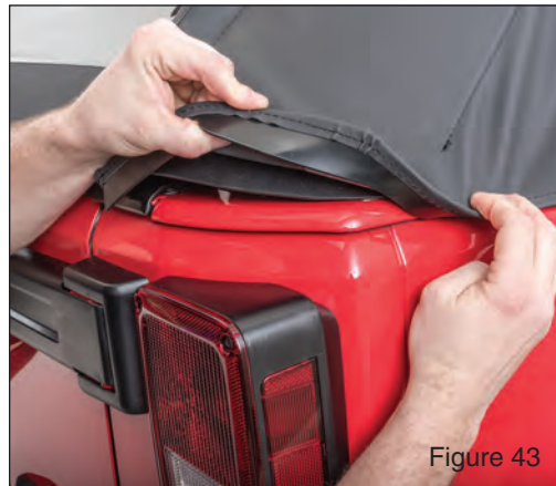
Figure 43 Work your way around the corners of the rear window. Starting from the side. (see FIG 43)
