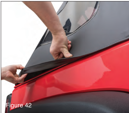
Figure 42 Slide lower window channel into body tub rail as shown. (see FIG 42)
