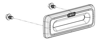
3. Reinstall winch hook. AEV recommends using the AEV Winch Hook Isolator (AEV80808014AA) to protect the fairlead.
