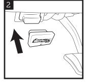
Insert ProCal SNAP into the OBDII port.
