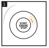
Press 2 times to put into the "RUN" position.
