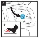
With your foot on the brake, PRESS and HOLD the CRUISE ON/OFF button for 3 SECONDS.
