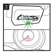
Wait for a blinking GREEN light on the SNAP and a blinking BRAKE light on the speedometer.
