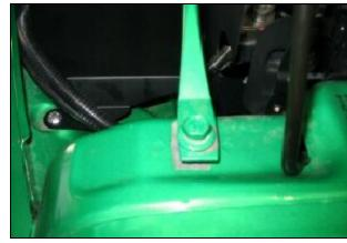
**12.** Using a ½" socket, reinstall the original bolt on the radiator support rod.
