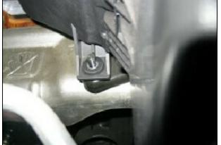
2. Loosen hose clamp attaching air filter assembly to throttle body. Using a ½" socket, remove bolt on back side of air filter assembly.
