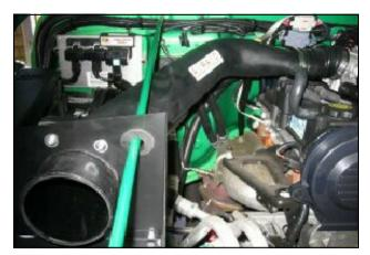
13. Install factory throttle body coupler on end of Airaid intake tube and position assembly on engine as shown. Mount Airaid intake tube to Cool Air Dam using two supplied ¼"-20 bolts and washers provided. Connect factory breather hose to Airaid intake tube.
