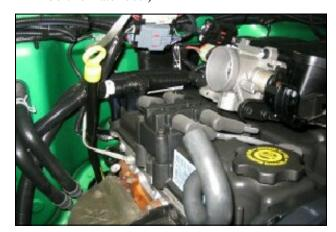
**4.** Remove air filter assembly from engine compartment. Retain rubber throttle body coupler for later use.
