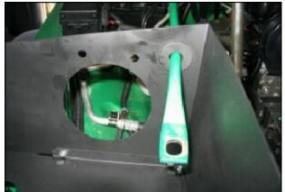
**8.** Position Airaid Cool Air Dam in place by inserting factory radiator support rod through grommet as shown.
