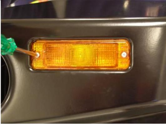
9. To install indicator lights to the bull bar, fit plastic plugs into the cavity in the wing and fix the light to the plastic plug from the front using screws supplied in indicator fitting kit.
