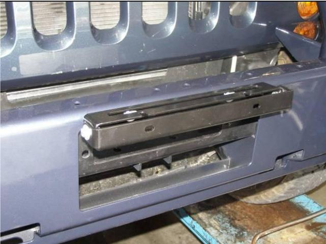
16. Mount number plate bracket assembly to bull bar using M6 fasteners supplied with number plate fitting kit.
