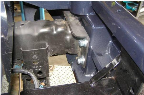
11. Loosely fasten bull bar to vehicle chassis using M10 fasteners supplied in chassis mounting kit.
