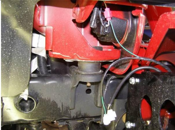
30. a) To wire the indicators to the RHS of vehicle, connect green wire (black trace) from bar loom to white wire (brown trace) from vehicle indicator. Secure using scotch lok.
