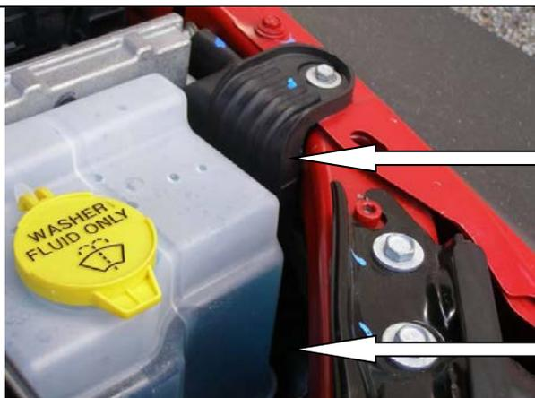
28. Feed loom under bracket and down between washer bottle and engine bay brace.
