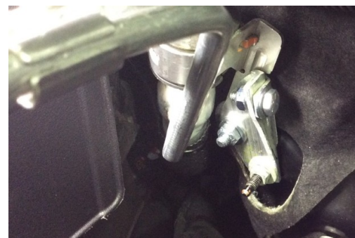
Modified location of Firewall bracket
