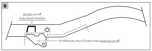
Use your new Safe-T-Cap<sup>TM</sup> as a guide and marker or chalk out a basic fit placement, then cut out frame 1" below the reference lines. Grind the remaining area clean and position the Safe-T-Cap<sup>TM</sup> in place with measurements referenced in illustration A.
