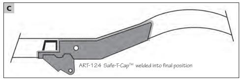
Fit the Safe-T-Cap<sup>™</sup> tight up into frame. Measure again and tack weld the corners. Once satisfied with final position and appearance, weld all edges 100% solid. Move your welds around to avoid possible overheating.
