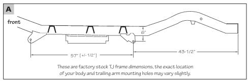
Start by measuring the distance between holes centers of the front and rear trailing arm mounts, be as accurate as possible and record for exact fit. These measurements are key for factory correct alignment of your new Safe-T-Cap $^{\text{TM}}$  and proper suspension performance.
