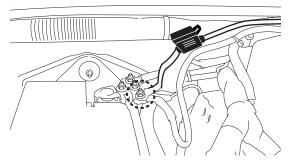
4 Route the power cable through the blank grommet on the firewall on the drivers side.
