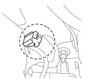
8 Remove (1) 10mm screws from under the each enclosure.
