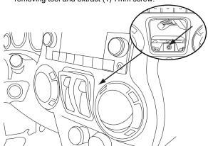
**5** Extract (4) 7mm screws and remove the factory radio.
