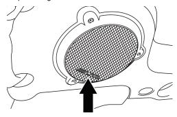
**8** Align the factory speaker grille over the tweeter bridge grille adapter tabs, connect the vehicle plug to the speaker and mount to the sound bar using the (3) T15 Torx screws.
