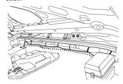
**5** Use the supplied cable ties to secure the main harness to the dashboard frame with the inductors between the vehicle's body and dash board frame.
