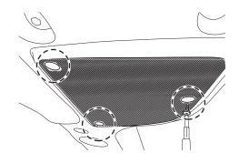
2. Remove (5) T20 Torx screws, disconnect and remove both speakers.
