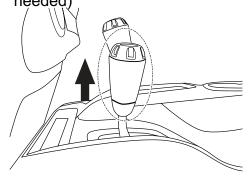
2 Remove the shifter panel by carefully pulling upward and releasing the clips with a panel removal/tooly
