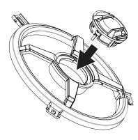
3 Route the wire through the notch on the basket, then press the grille into place. Ensure the wires do not get pinched.
