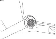
2 Gently open the (3) lock tabs to release the factory tweeter.
