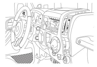
6 Extract (4) 7mm screws and remove the instrument cluster.
