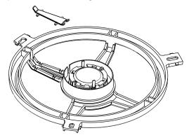
4 Add foam strip on top of wires in channel.
