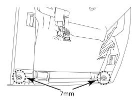
**5** Remove glove box by pushing both left and right sides inwards.
