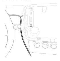
**10** Mount the bass level knob in one of the suggested locations. Use a drill bit size 9/32".
