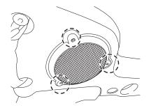
2. Disconnect and remove the factory speaker.
