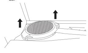
2 Using a 7mm socket remove (2) screws, disconnect and remove the factory speakers.
