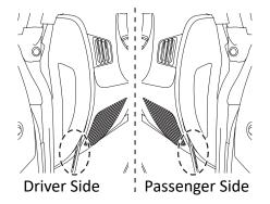
2 Remove the driver side knee cover by releasing the (2) top clips.
