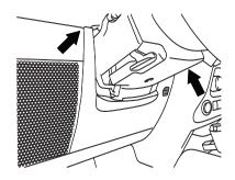
3 Extract (2) 10mm screws from the metal steering wheel column cover and remove it.
