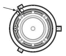
Select the (2011-2014) crossover input wires and connect to the vehicle plug. Connect tweeter connectors. Secure the crossover. Note: 2015-2017 input plug is not used.
