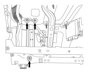
14 Connect both amplifiers Note: Be sure to insert the corresponding connector into each amplifier.
