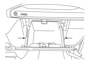
**6** Extract (2) 7mm screws located on the lower dash section.
