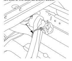
4 Place the passenger seat over the enclosure while carefully aligning the enclosure in between the seat rails. Mount using (4) 18mm seat bolts.
