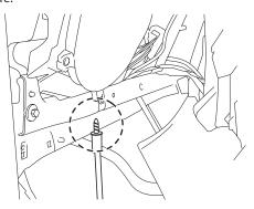
10 Pull the dash towards the back of the vehicle and remove the enclosure by turning towards the back.
