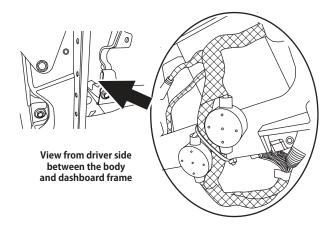
2 Use a 10mm socket to connect the power cable to the POSITIVE (+) battery terminal. Note: The NEGATIVE terminal should remain disconnected until the installation is completed.
