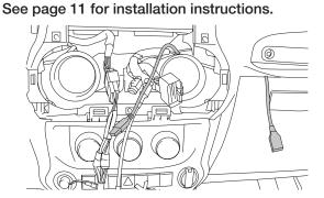
6 Route the key harness through the top-left side of the i209 source unit. Mount the i209 source unit using (4) 7mm factory screws.
