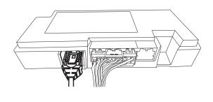
3 Connect the 4pin OEM connector to the OEM USB adaptor (included).
