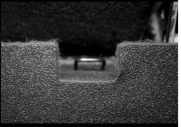
Pre-drill all holes through the existing holes in the Armorlite seatback cover using a 1/8" drill bit. Leave the seatback cover in position and drive screws by hand with provided fastener screws. **IMPORTANT:** do not use a larger sized drill bit. This could cause screws to not fit properly and come out over time.
