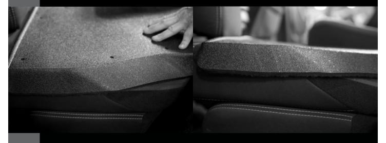
The Armorlite pre-drilled fastener holes need to align over the internal metal frame found at the top of the back seat. Holes will be drilled directly into the seat frame.
