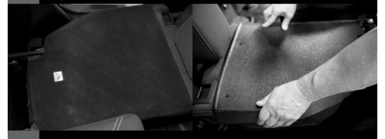
Take the driver side Armorlite seatback cover (40% / smaller piece) and place the left outside wall over the back seat so it is flushed with the side cushion of the seat.
