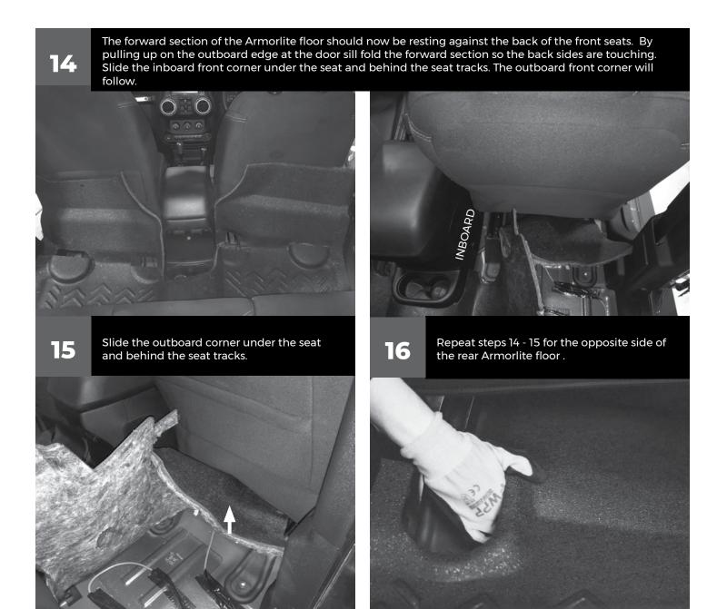
Tuck the outboard edge under the door sill. Ensure that the floor is tucked under the trim at the "B" pillar and NOT against the trim. This will result in an improper fit and the drain holes will not align.
