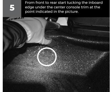
Tuck the rear, inboard part tail under and between the seat track and center console trim.
