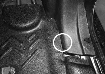
Ensure the rear Armorlite floor is on top of the front Armorlite floor, and the seat wires are properly routed through the slots and holes.
