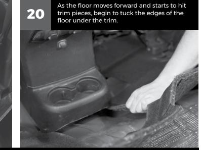
Repeat steps 19 and 20, by alternating sides until the rear Armorlite floor is in the correct position. Use the drain hole as a reference.
