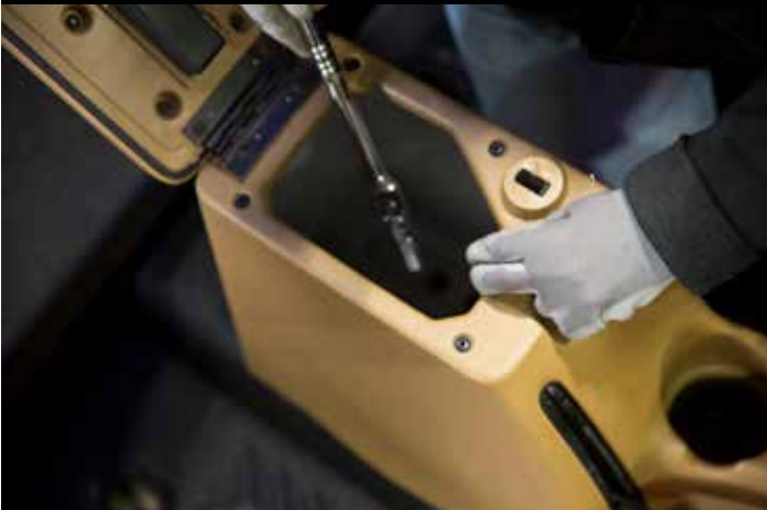
2 - M10 bolts inside storage bin
