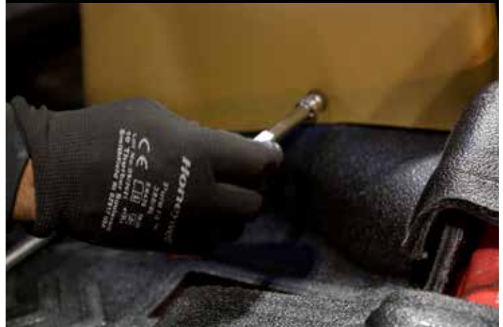
2 - M10 bolts on outer passenger side wall of storage bin
