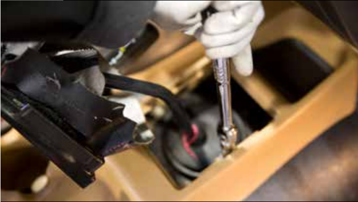
1 - M10 bolt under shift panel
