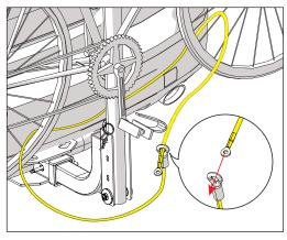
Weave the cable through the bike frame, wheels, etc. and then pass the small steel eyelet through the cable loop.
