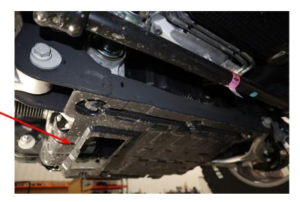
With the stock skid plate removed, you can now see the bolt locations for your new LOD skid plate on the front frame crossmember. You will also need to remove one the frame bolts that mount your front differential.
