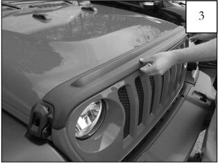
Center the part on hood. Part should be about 1/16" from hood edge on all sides.
