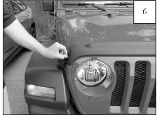
Again using the same process, remove tape liner from passenger side Far Side Edge of hood proector. Repeat for passenger side.
