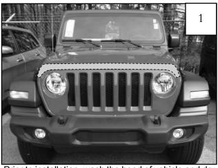
Prior to installation, wash the hood of vehicle and dry with a clean cloth. Use the alchohol pads to clean entire LEADING EDGE of hood. *NOTE: Temperature should be at least 60°F for proper tape adhesion.*
