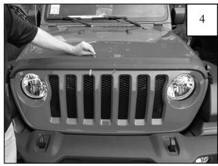
Begin removing tape liner starting with the passenger side Center Top. Grasp the free end and pull tape gently in 6" sections. Apply even pressure with opposite hand to the hood protector while pulling tape liner. Repeat for driver side. **NOTE:** You must apply even pressure from center section out to each end of part for proper adhesion to hood.
