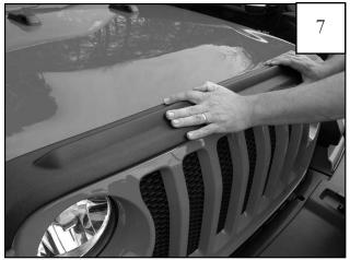
Apply firm pressure along all edges of hood protector to ensure adhesion of tape to hood surface. Installation is now complete.
