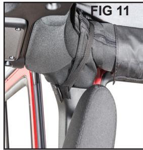
**Step 4: Install side tension straps**
