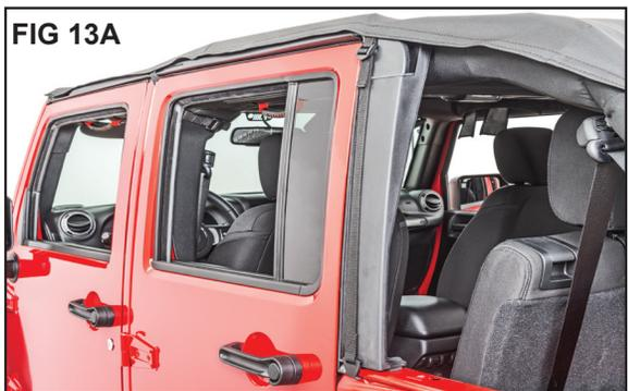
**Step 6: Install long side tension straps.**
