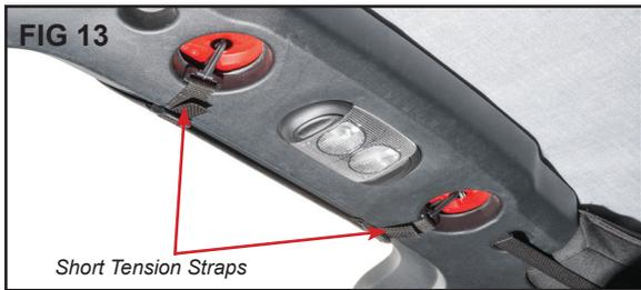
**Step 5: Install short tension straps**
