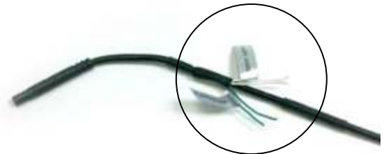
Green and white wires on the camera harness.
