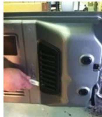
8. Pull the harness through the rear gate openings
