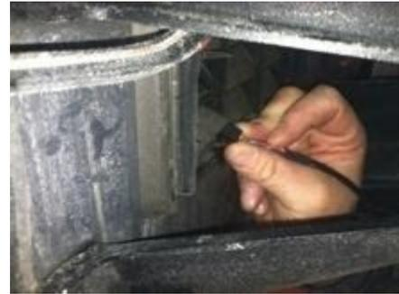
7. Using a plastic trim removal tool, remove interior panels on the inside of the rear gate.
