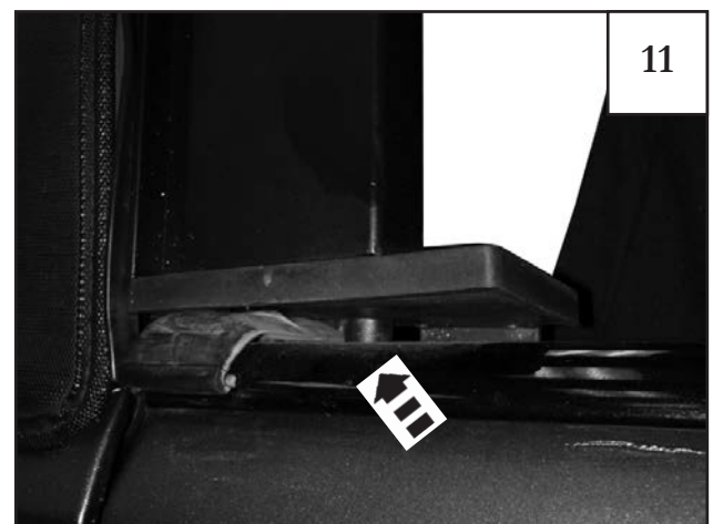
Position completed door surround onto the vehicle and fit the bottom base pin into the hole in vehicle tub near the rear door latch.
