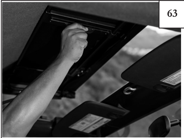
Grab the Flip Top Center Grab Handle and push up. The frame will pivot towards the back of the vehicle and rest on itself.
