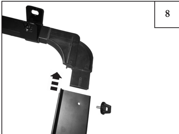
Insert the other end of the plastic corner part into the vertical extrusion part and secure with the turn knob screw.
