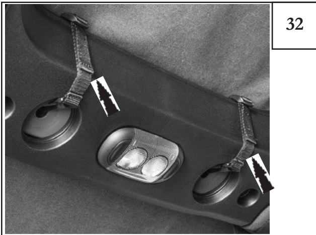
Wrap the two straps attached to the middle section of fabric around the rear-middle of the sound bar.
