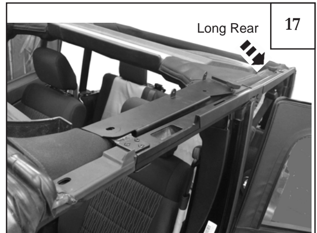
Starting at the driver side rear bracket hole insert door surround knob Long Rear (LR) 2.75" into hole and tighten.
