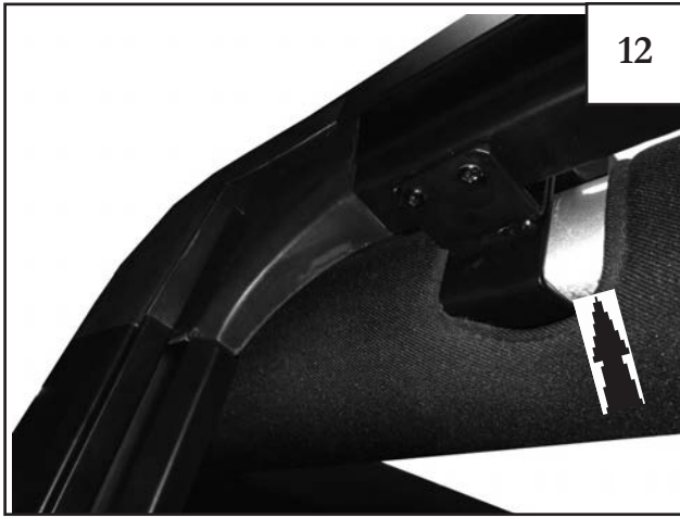
Position completed door surround rear bracket onto the vehicle and fit the bracket over the sport bar.
