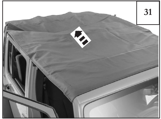
Un-Fold the soft top over the sport bar frame working toward the rear of vehicle.
