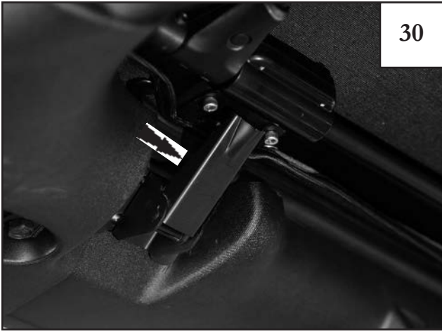
Closed and secure the front latches as shown on both sides at this time.
