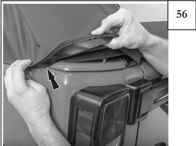
Work your way around the corners of the rear window. Starting from the side.
