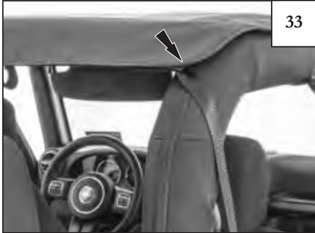
Locate the long strap at the rear corner of the main deck. Pull it straight and to the outside of the sport bar.
