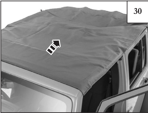
Un-Fold the soft top over the sport bar frame working toward the rear of vehicle.
