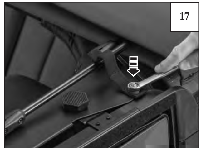
Put the retention strap in place with the bolt through the grommet as shown. Next, install the 2nd washer and Nylock nut on top of the strap and tighten with 13mm socket wrench and 13mm wrench.
