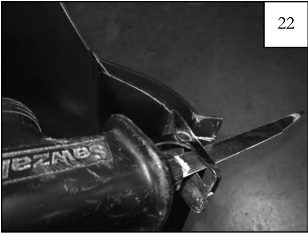
Using a sawsall, cut of section marked in step 21.
