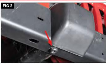
Put on safety glasses. Using a T55 torx bit driver or socket remove the tow hooks and/or bumper bolts. (Fig 1) Repeat the step for the other side. Remove the lower bumper bolts with and T55 torx bit driver or socket. (Fig 2) Repeat the step for the other side. Remove the factory bumper.
