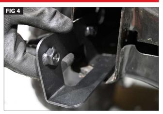
If equipped, remove the three bolts attaching the original recovery hook using a 18mm socket. Recovery hook will not be reused with the new rear bumper. (Fig 3) On the passenger side and drivers side, insert the supplied M12 nut plate into the frame rail. Align the threaded holes in the nut plate with the holes in the frame on the side. (Fig 4)
