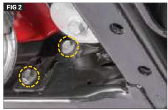
Put on Gloves and Safety Glasses. Open tailgate. Swing it so that spare tire is out of the way. Remove the (4) M10 bolts (2 per side) that attach the rear bumper brackets to frame using a 16mm socket. (Fig 1) Remove the (4) M10 bolts holding the rear bumper support brackets frame using a 16mm socket. (Fig 2) Remove the brackets and bumper from the vehicle.
