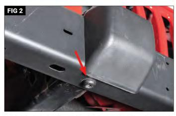
Put on safety glasses. Using a T55 torx bit driver or socket remove the tow hooks and/or bumper bolts. (Fig 1) Repeat the step for the other side. Remove the lower bumper bolts with and T55 torx bit driver or socket. (Fig 2) Repeat the step for the other side. Remove the factory bumper.
