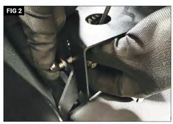
Use the stone guard to mount optional lighting behind the perforated screen in the bumper. With the connecting harness for the light through the wiring hole of the stone guard, insert the mounting bolt from the light into the tab on the bumper behind the screen. (Fig 1) Place a flat washer and nut onto the bolt. (Fig 2) Do not fully tighten.
