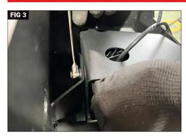
Once auxiliary light is aimed as desired, tighten bolt as needed. (Fig 3) Repeat the step for other side.
