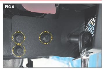
With the assistance of another person, and with the tailgate partially open, lift the bumper and gently rest it on the frame rails. Attach the bumper to the frame. (Fig 5) Install the passenger side using the supplied bolts with a 18mm and 16mm socket. (Fig 6) Snug the bolts first. Align the bumper, then tighten the factory side mounting bolts on both sides. Torque all mounting hardware to 105ft-lbs. Installation is now complete.
