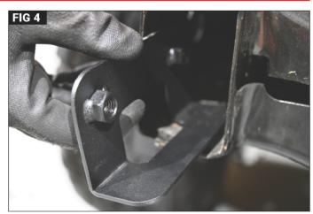
If equipped, remove the three bolts attaching the original recovery hook using a 18mm socket. Recovery hook will not be reused with the new rear bumper. (Fig 3) On the passenger side and drivers side, insert the supplied M12 nut plate into the frame rail. Align the threaded holes in the nut plate with the holes in the frame on the side. (Fig 4)
