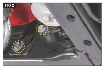
Put on safety glasses. Open tailgate. Swing it so that spare tire is out of the way. Remove the (4) M10 bolts (2 per side) that attach the rear bumper brackets to frame using a 16mm socket. (Fig 1) Remove the (4) M10 bolts holding the rear bumper support brackets frame using a 16mm socket. (Fig 2) Remove the brackets and bumper from the vehicle.
