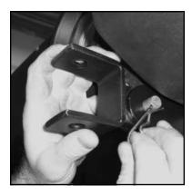
11) Attatch tow bar ends by inserting them into the bracket on the plate and affixing them in place with the clevis pins and hairpins. Tow bar ends must then be bolted to the tow bar of your choice.
