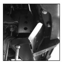
**8)** Install the remaining 2 top bolts, using the 3/8"-24 x 1" bolts, a washer top and bottom, and the nylock nuts. Go ahead and tighten these bolts down.
