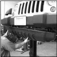
1) Remove all plastic attaching screws from stock plastic valance panel, then remove the panel from the vehicle.
