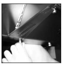
**9)** Start several of the bottom bolts into their holes with washers and nuts, and then remove the C-clamp or Vise-Grips that you had the plate clamped to the crossmember with.
