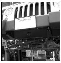
4) Before proceeding any further, center the new plate side to side on the vehicle using the bumper guards and the tow bar mounts on the plate as reference. Tighten the 4 top bolts.
