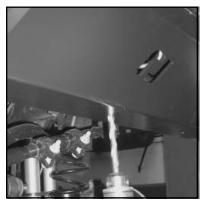
7) Now go back and drill the holes. Drill pilot holes first with a 3/16" bit, and then follow that up with a 3/8" bit.
