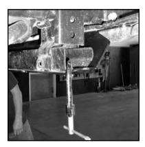
**5)** Next, with C-clamps or Vise-Grips, clamp the back of the plate up snuggly to the bottom of the crossmember.
