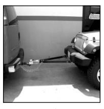
**12)** For optimum performance your tow vehicle's hitch should allow for the tow bar to ride as level as possible. Always use safety chains (included with the CE-9033F tow bar). This system will work with universal adjustable tow bars from Friedl, Draw-Tite, Valley, or Blue Ox.
