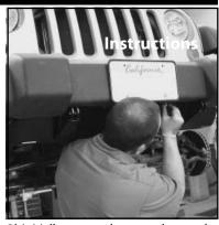
**3)** Initially mount the new plate to the bottom of the bumper by installing 4 of the 3/8"-24 x 1" bolts, washers top and bottom, and nylock nuts in the 4 pre-existing upper holes. Snug these bolts, but do not tighten.
