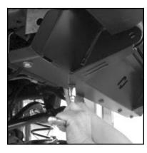
**10)** After all of the lower bolts are in their holes, go back and tighten all of the bolts with a 9/16" wrench on top and socket on the bottom.
