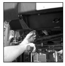
**6)** Using the plate as a template, and a 3/8" transfer punch, punch the 2 undrilled upper holes and all of the bottom holes.
