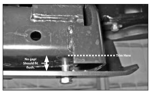
**Update!** We have found on 2010 and up models that the front crossmember has changed! As you can see in the photo, the vertical frame beam now overhangs the bottom of the crossmember that the tow bar plate mounts to. We have found that the easiest way to fix this is cut the bottom of the vertical beam off flush with the crossmember allowing the plate to fit flush against the crossmember.
