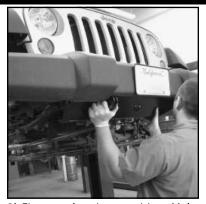
2) Fit new plate into position. Make sure the ends of the new plate wedge between the ends of the stock plastic bumper cover and the metal of the frame crossmember.
