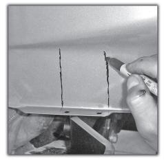
**17)** Next, with an arm installed, mark your trim area to be cut out. This should be centered around the arm, and about 2 1/4" wide and 3 1/2" tall.
