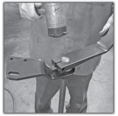
**3)** Install the right hand side bracket onto the end of the sway bar with a mallet just far enough that the face of the arm is flush with the end of the bar.
