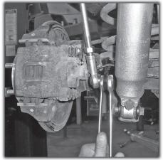
**31)** After you are satisfied with the shock and heim joint fitment, go ahead and tighten ONE of the heim joints down. Run the nut down on the opposite one, but do not snug or tighten it at this time.
