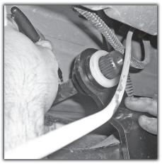
6) If your vehicle does not have a body lift, like our subject vehicle here, it will be necessary to mark the body tub flange in the location where the sway bar contacts it so that clearance notches can be ground on both sides.
