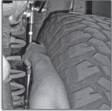
**33)** Adjust the link that you left untightened in step 31 until the studs in the heim joints are completely neutral. As in - the studs are both parallel to the ground and can slide in and out of their bolt holes with no bind.
