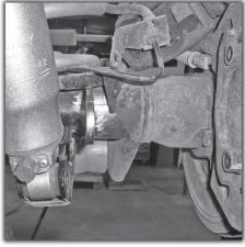
**25)** Our subject vehicle had the shock mounts replaced at one time, and this is where optimum tab location fell in this instance. We will be running our link heim joints on the outboard or tire side of the housing tabs.
