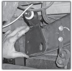
**5)** Align the slotted hole in the bracket with the large hole in the frame. Raise the or lower the bracket based on the slotted hole until the sway bar is clear of the gas tank.
