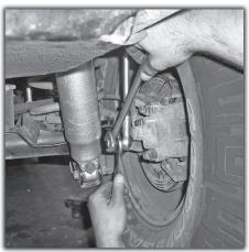
**34)** With the link adjusted, you may finish the tightening of the nut that you had left loose. Check all of the other hardware that you've installed or disturbed during this intsallation to make sure that it is reinstalled and torgued to standard specs.
