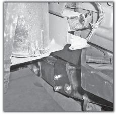
**19)** This is what the sway bar arm interference should look like on the passenger's side before trimming. This area will appear different on early TJ's that did not have the charcoal canister in this location.
