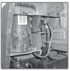
**20)** Articulate the arm upward and trim the sheetmetal on the charcoal canister brackets as necessary. When you are finished it should look like this.
