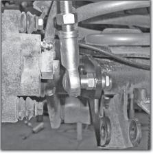
**30)** Full nyloc nuts and thin nyloc nuts are supplied in the kit. In this application, after the heim joint threads were trimmed, the thin nyloc nut is used as opposed to the full nyloc.
