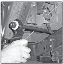
**4)** Slide the bar through the back of the vehicle from the passenger's side as shown. Be mindful of wiring and lines in this process!!!
