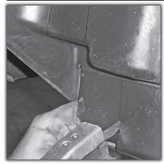
**22)** Trim your plastic inner fender panels accordingly. Again, you may use a saws-all, jig saw, or tin snips - we used an air hack saw.
