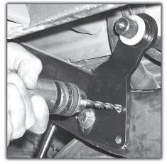
**14)** Center punch all 4 of the small holes with a 3/8" transfer punch, pilot drill, and then drill with a 5/16" drill bit.
