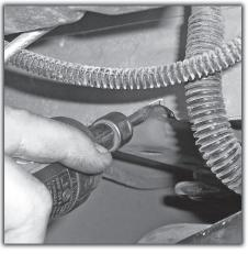
**9)** Grind notches in the tub flange for sway bar clearance.
