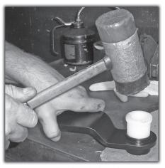
**2)** Using a mallet, knock the white UHMW bushings into the frame brackets. Take note of the bushing flange, and the "Z" in the bracket when installing.
