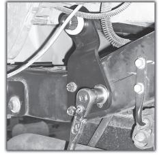
**16)** After a final fitment check, go back and tighten ALL SIX bolts.
