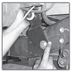
**13)** Raise, lower, and or rotate the bracket as needed before center-punching the 2 smaller holes.
