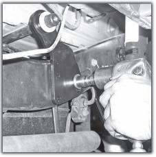
**12)** Insert the other 1/2" flat washer and 1/2" stover nut on the inside of the frame rail. Snug bolt down but do not tighten!
