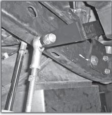
**28)** Assemble the end links, if you haven't already, with an initial setting of 16" from center of rod end stud to center of rod end stud. Install them in the holes in the arms and tighten them down. The nut goes on the tire side of the arm.
