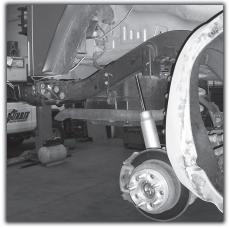
1) After removing the rear wheels & tires, remove the plastic rivits that retain the back ends of the plastic inner wheelwells to the body tub. Lower the panels down out of the way.
