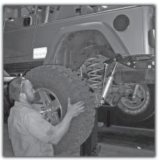
**33)** You may now reinstall your wheels & tires and set the vehicle back down on the ground so that final adjustments can be made at ride height with the weight on the suspension.
