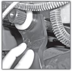
**10)** Align the slotted hole in bracket with the large hole in the frame again to check your clearance. Grind the notchesmore if necessary.
