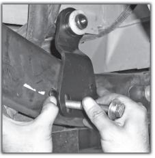
**11)** Install the driver's side bracket and then, on both sides, install the tube spacer through the hole in the frame, and insert the  $1/2^{"} \times 4^{"}$  bolt with washer thru the bracket and the tube spacer.
