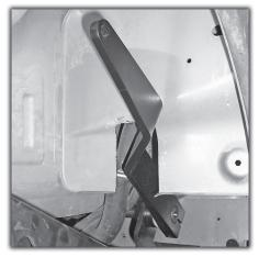
**18)** Cut out the trim area with a saws-all, jig saw, or tin snips. We used an air hack saw. Then test fit the arm clearance to make sure it is sufficient.
