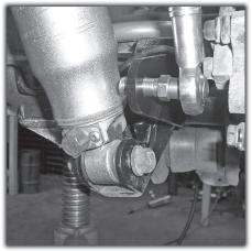
**29)** Again in an effort to present this in as "real world" of a fashion as possible, where you may have bought a used vehicle with modified shock mounts, we are able to illustrate here that this shock mount combination will require trimming of the heim joint threads.
