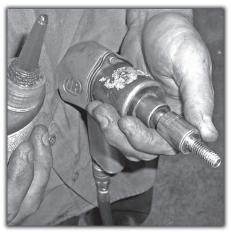
**15)** Put red loc-tite on the 4 thread rolling bolts and run them into the holes.
