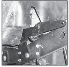
**23)** Test fit the inner panels and when when you are satisfied with the fit, reattach them to the tub using their plastic riviets.
