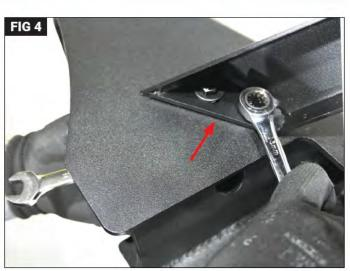
Align the Carnivore over ride bar with the corresponding holes of the Carnivore front bumper and install using two M8 - 1.25 x 25mm Bolts, two flat M8 washers, two M8 lock washers, and two M8 nylock nuts. (FIG 3) Tighten each bolt with a 13mm wrench and socket. (FIG 4)
