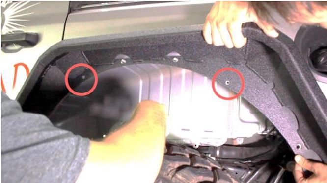
With a 13mm wrench and 5mm Allen key, tighten down the bolts. Repeat on the opposite side.
