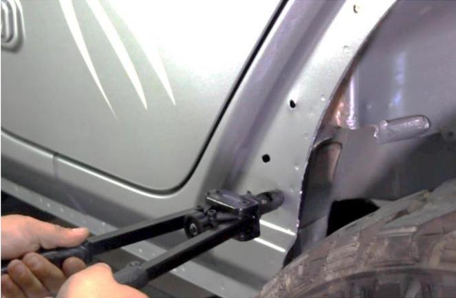
With the bolts still loose, push the turn signal power cord between the body and fender brackets.
