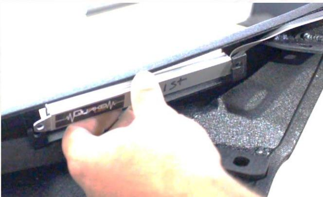
Secure the signals to the fender using a 3mm Allen wrench with the included M5 bolts, washers, and serrated nuts.
