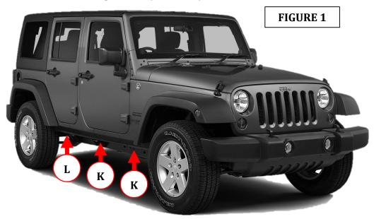
**Step-1** Begin the installation on the passenger side. Starting at the front of the vehicle, locate the holes in the body pinch mold and in the underside of the body, (FIGURE 2).
