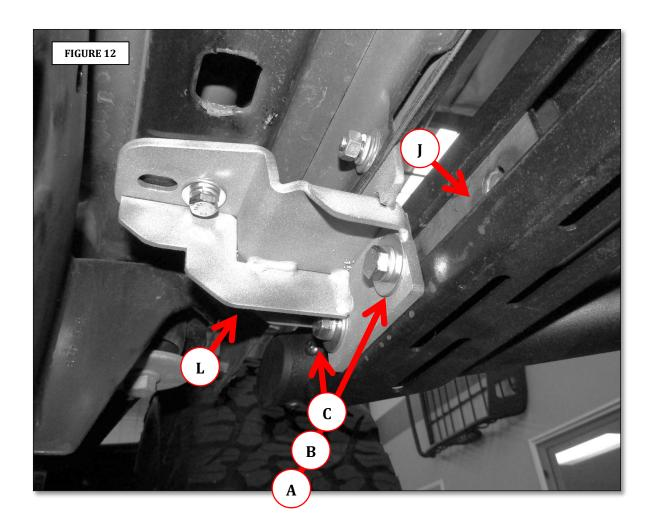
**Step-9** Align the Dominator D6 Side Step with the vehicle and tighten all bracket and side step nuts and bolts,. Repeat the above steps to install the brackets and Dominator D6 Side Step on the driver side of the vehicle. Remember to check and retighten the nuts and bolts every six months.
