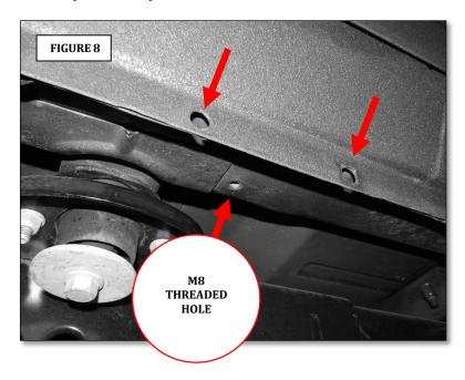
**Step-6** Attach the passenger side rear bracket to the pinch mold using (2) 5/16" x 1" button head bolts, (2) 5/16" flat washers, (2) 5/16" lock washers and (2) 5/16" hex nuts, and to the underside of the body using (1) M8 x 25mm hex bolt, (1) 5/16" lock washer and (1) 5/16" flat washer, (FIGURE 9 & 10). Leave the nuts and bolts loose for final adjustment.
